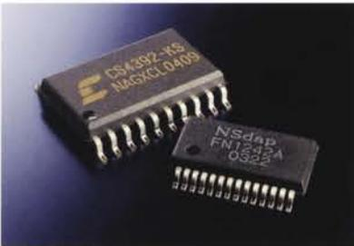
This is the sound quality of stereo reproduction considered as the highest frequency in the listening environment of audio file. As for front L/R output, the "FE type DAC" (FN1242A), which could be called the aesthetic consciousness of Luxman is driven with the
