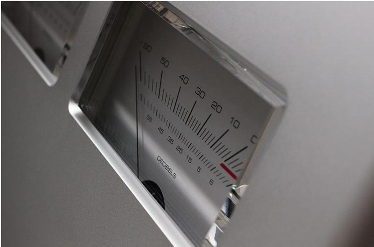
At the center and right of the upper half of the M-900u's front panel are two power meters, to indicate how hard the M-900u is working and to add a bit of retro styling and pizzazz, 1970s style. The beveled glass covering the meters, of the same look and quality as the one
